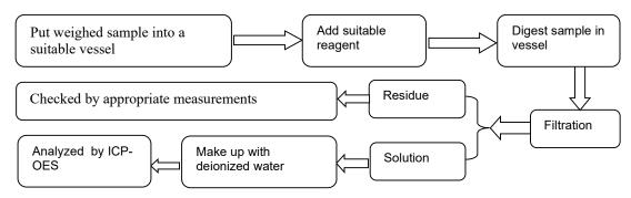
2. Test for Mercury (Hg) contents (IEC 62321-4:2013/AMD1:2017):
